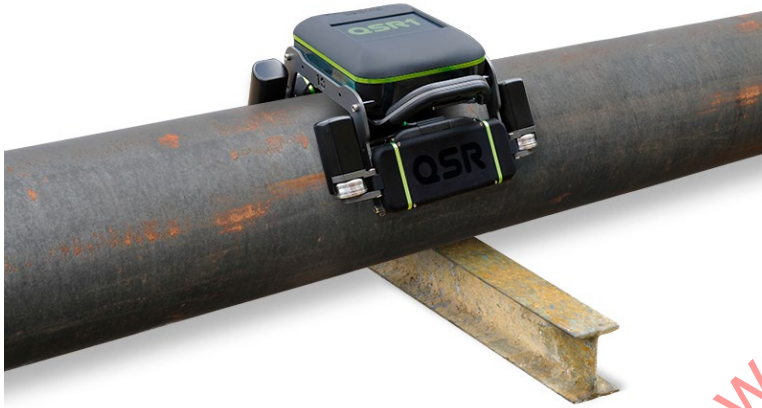
Mechanized EMAT with qualitative thickness measurement
